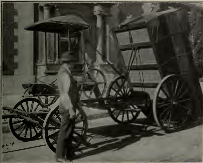
ONE MAN CAN READILY DUMP THIS BODY
